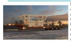
For an injured employee who cannot walk off of a vessel via the gangway, a Hustler will retrieve the rescue cage via MAFI and bring it to the crane. A forklift may also be used. After locking the spreader bar into the corner castings and connecting the 4 safety chains to the spreader bar, the Cage may be used to transport employees to/from the vessel.
