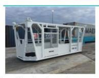
For an injured employee who cannot walk off of a vessel via the gangway, A Straddle Carrier/ Shuttle Truck will retrieve the rescue cage and bring it to the crane. After locking the spreader bar into the corner castings and connecting the 4 safety chains to the spreader bar, the Cage may be used to transport employees to/from the vessel.
