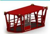
For an injured employee who cannot egress a vessel via the gangway, a straddle carrier/shuttle truck will retrieve the rescue cage and bring it to the working crane. After locking the spreader bar into the corner castings, and connecting the 4 safety chains to the spreader bar, the cage may be used to transport employees to/from the vessel.
